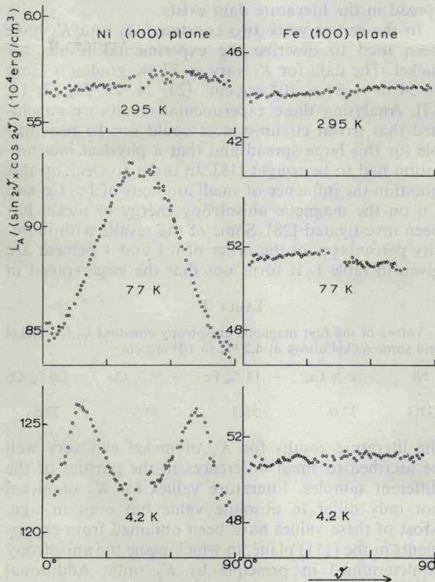
FIG. 1. — Higher order contributions to the torque curves of Ni and Fe in the (100) plane. In order to eliminate contributions from  $K_1$  to the angle dependence, the experimental data have been multiplied with the factor  $(\sin 2\theta_i \times \cos 2\theta_i)^{-1}$ . (After ref. [15] and [18]).
